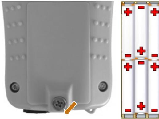
**WARNING: BATTERIES MUST BE INSTALLED AS PICTURED ABOVE TO AVOID EXCESSIVE HEAT OR PERMANENT DAMAGE TO THE READER DURING CHARGING**
