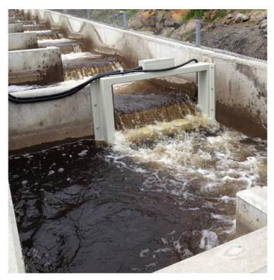
The Biomark **FISH PASSAGE** Antennas are typically designed for the specific application or site. Antennas are fully submersible and can be used to monitor Ice Harbor style weirs, with overflow and submerged orifices or antennas can be integrated into vertical slots or sample the entire passage channel. Antennas are typically constructed with internal or external shields to mitigate for potential electromagnetic interference.
